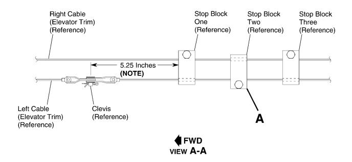
**NOTE:** Make sure that the elevator and the trim tab are in the neutral position when Stop Block One is installed.
